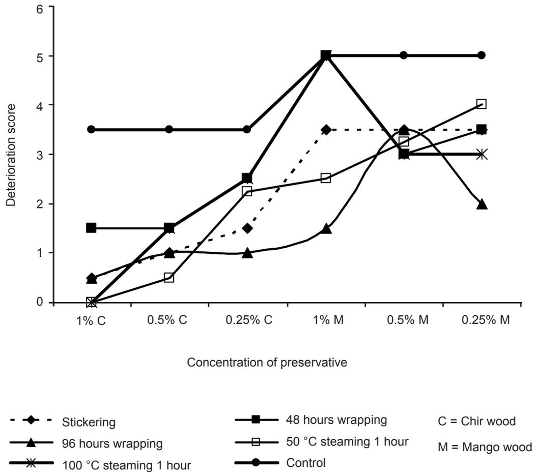
Figure 2 Deterioration of chir and mango wood in the field
