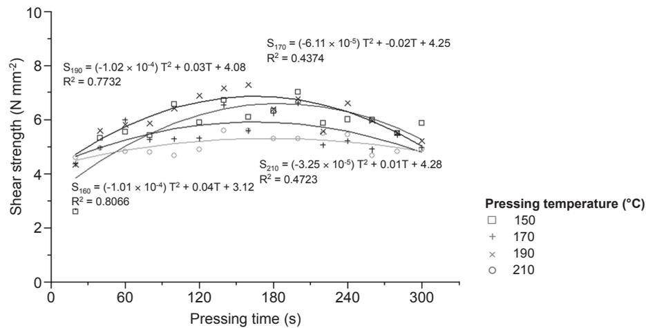
Figure 5 Shear strength of PF-glued bamboo strands as a function of pressing time and temperature
