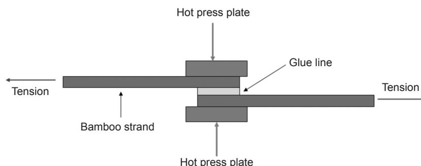
**Figure 1** Schematic description of shear test by Automated Bonding Evaluation System (ABES)
