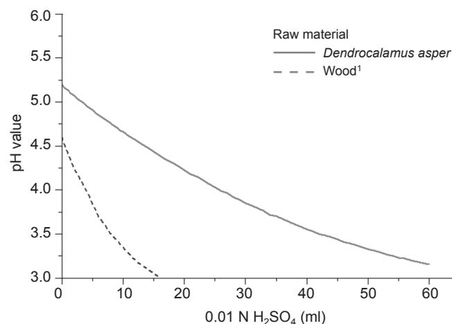
**Figure 2** pH changes of *Dendrocalamus asper* and wood during acid addition; <sup>1</sup>Sauter (1996)
