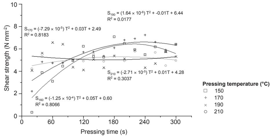
Figure 4 Shear strength of MUPF-glued bamboo strands as a function of pressing time and temperature
