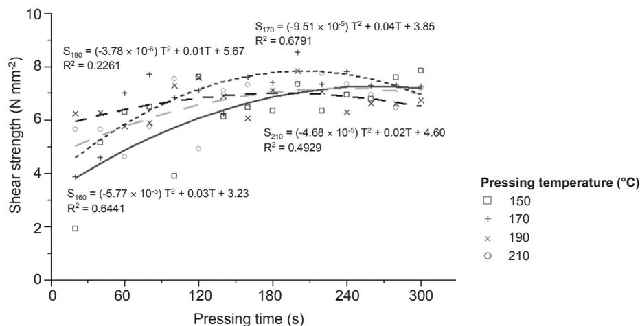
**Figure 3** Shear strength of MF-glued bamboo strands as a function of pressing time and temperature
