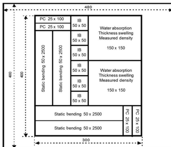
**Figure 1** Distribution of the specimens in sample particleboards; PC = parallel compression, IB = internal bond; measurements are in mm
