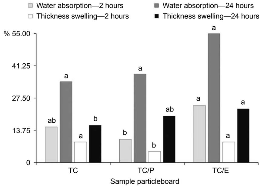
**Figure 5** Physical properties of the particleboards in stage 2; TC = 100% *T. ciliata*, TC/P = 50% *T. ciliata* + 50% *P. oocarpa*, TC/E = 50% *T. ciliata* + 50% *E. grandis* × *urophylla*; means followed by the same letter do not differ at  $p < 0.05$
