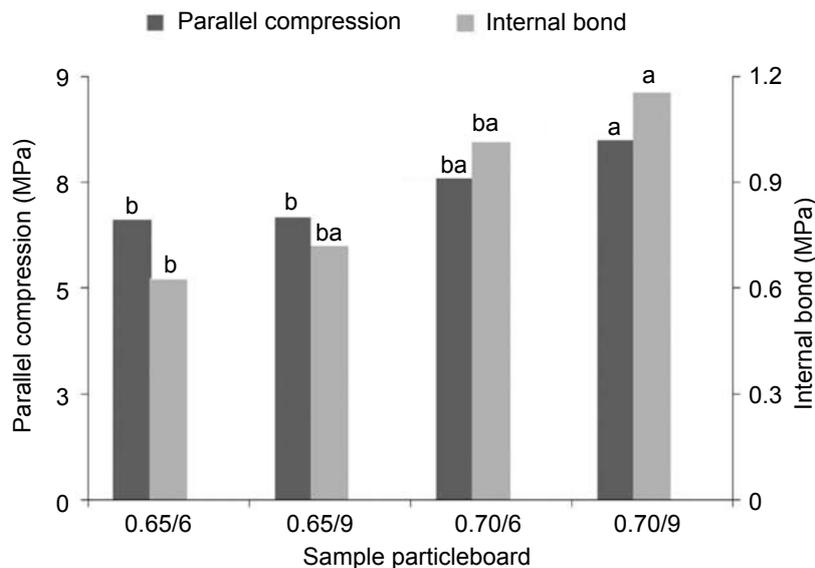
**Figure 4** Parallel compression and internal bond of particleboards in stage 1 (100% *Toona ciliata*); details of samples are as in Table 1; means followed by the same letter do not differ at  $p < 0.05$
