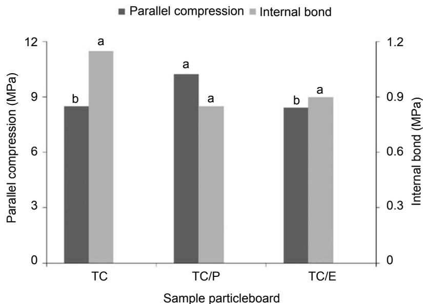
**Figure 7** Parallel compression and internal bond of the particleboards in stage 2; TC = 100% *T. ciliata*, TC/P = 50% *T. ciliata* + 50% *P. oocarpa*, TC/E = 50% *T. ciliata* + 50% *E. grandis* × *urophylla*; means followed by the same letter do not differ at  $p < 0.05$
