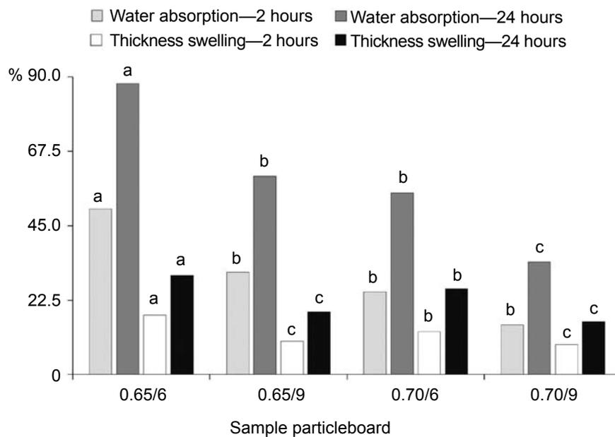
**Figure 2** Physical properties of the particleboards in stage 1 (100% *Toona ciliata*); details of samples are as in Table 1; means followed by the same letter do not differ at p < 0.05
