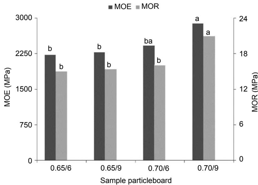
**Figure 3** MOE and MOR of the particleboards in stage 1 (100% *Toona ciliata*); details of samples are as in Table 1; means followed by the same letter do not differ at  $p < 0.05$
