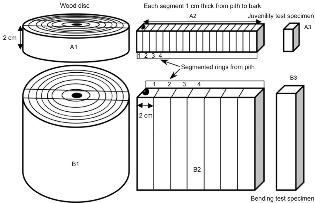
**Figure 1** Schematic drawing of the preparation of the juvenility and bending test specimens (Darmawan et al. 2013)
