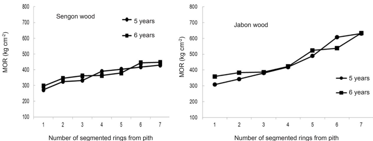
**Figure 6** Comparison of radial variation of average modulus of rupture (MOR) in 5 and 6-years old sengon and jabon
