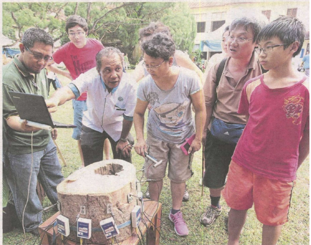
Green education: Dr Abdul Latif (second from left) and FRIM research officer Ahmad Azaruddin Mohd Noor (left) briefing visitors on how the Picus Sonic Tomography device is used.
