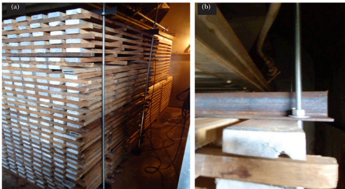
Figure 1 Endless screw for daily adjustment during drying, (a) endless screw location in lumber stacked in piles and (b) nuts and washer
